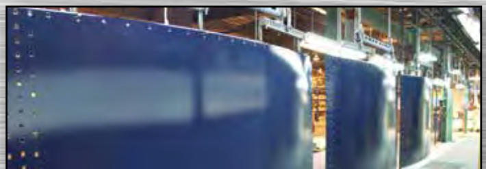
Stage 4: Glass-fused-to-steel sheets are quality tested and prepared for shipment
