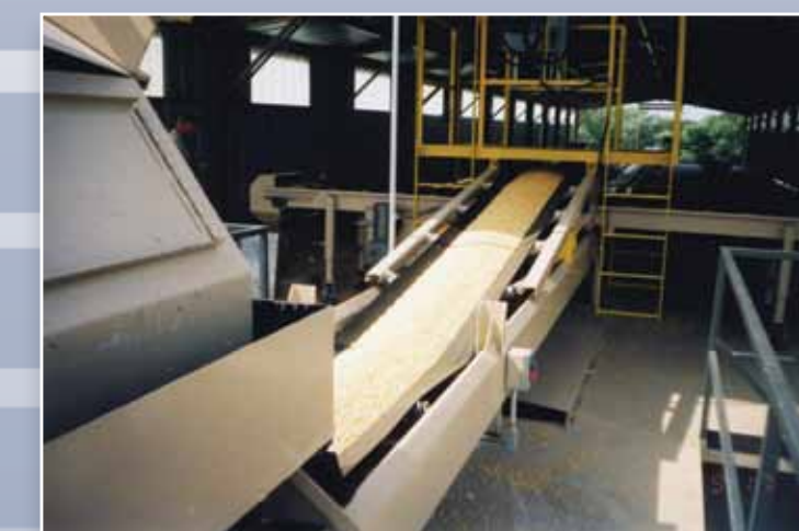
CROSS BELT TRIPPERS ✦ Designed for left or right powered discharge for stockpiling, bunker, or bin filling operations.
