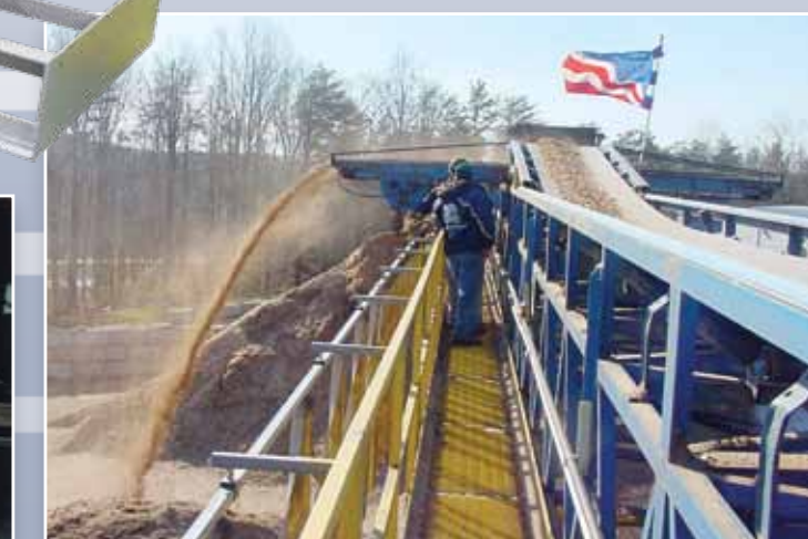
CROSS BELT TRIPPERS ✦ Designed for left or right powered discharge for stockpiling, bunker, or bin filling operations.
