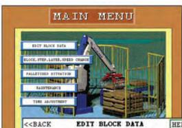
User friendly touch screen (HMI) with software that is specific for Palletizing.
