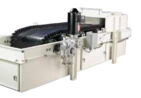
The Tecweigh WF18 sanitary weigh belt feeder is a stainless steel, wash-down duty weigh belt that has proven track record in a variety of industries including food, pharmaceutical and chemicals. The WF18 is designed to meet FDA and USDA standards featuring welded 304 stainless steel construction and provides product flow rates up to 250,000 pounds per hour.
